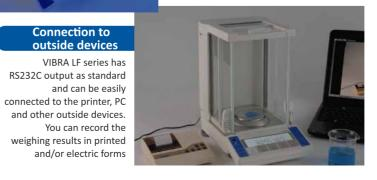
The laboratory/factory environment is changing every moment, and it affects the conditions of balance. In  $\alpha$ -check system, VIBRA LF series gives diagnosis menu of its own conditions. Among check-items repeatability is the most fundamental parameter in laboratory balance, and the user can easily check it in this system.
